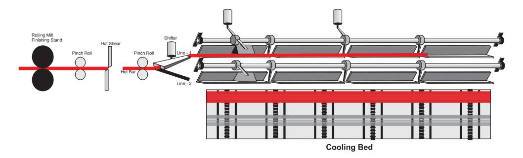
'Auto Twin Angle with Tail Breaker' features a bar handling mechanism used to collect TMT Bars and profiles like rounds / squares / hexagon upto 50 mm dia. It is a complete PLC controlled mechanism starting from shearing operation till the collection, breaking and dropping of the bars onto the cooling bed.
